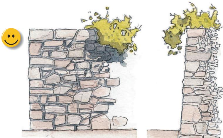
FIG. 1 - MURO DI SOSTEGNO IN PIETRAME SBOZZATO, A SECCO
